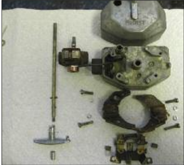
Photo 1 - Exploded View of Motor
