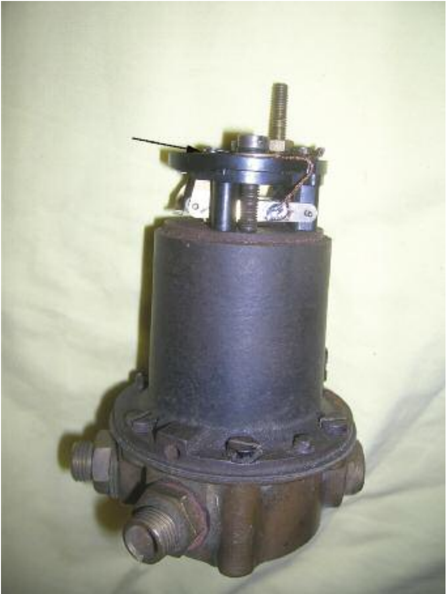
Fig 1: Spring contact over-travel gap to the housing top
