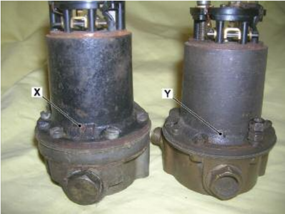
Fig 3: SU fuel pumps showing diaphragm failure vent holes
