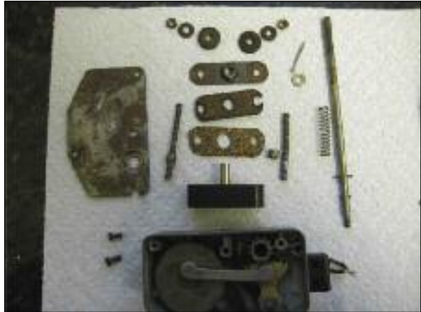
Photo 4 - Exploded view of Front (Gearbox side)
